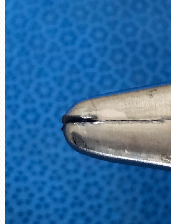
Damaged rongeur that was used to remove a pin
